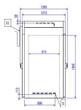
Drain Electrical inlet (power) RO Refrigerant Outlet
